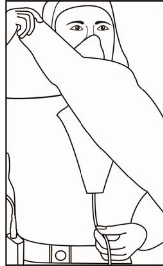
Fig. 6: Routing cable beneath inner shroud.
